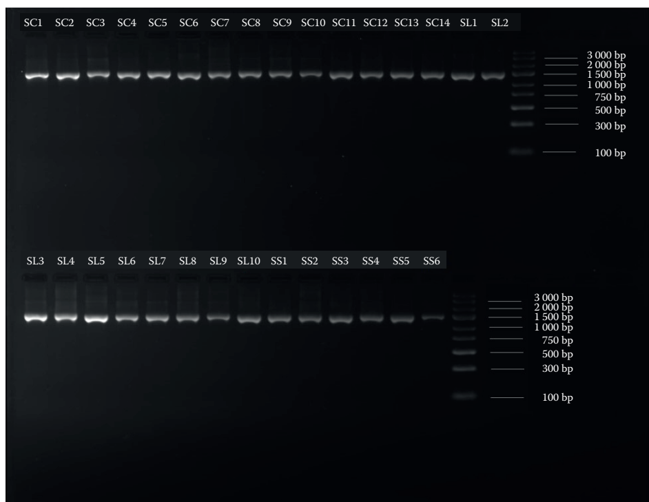
Figure 1. Electrophoresis gel with the PCR final products in connection to tested LAB isolates LAB – lactic acid bacteria; PCR – polymerase chain reaction; SC – 'sucuk'; SL – salami; SS – sausage
