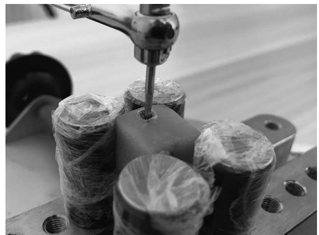
FIGURE 2. Reverse torque analysis of the titanium implants (Tonichi STC400CN, Buffalo Grove, IL).
