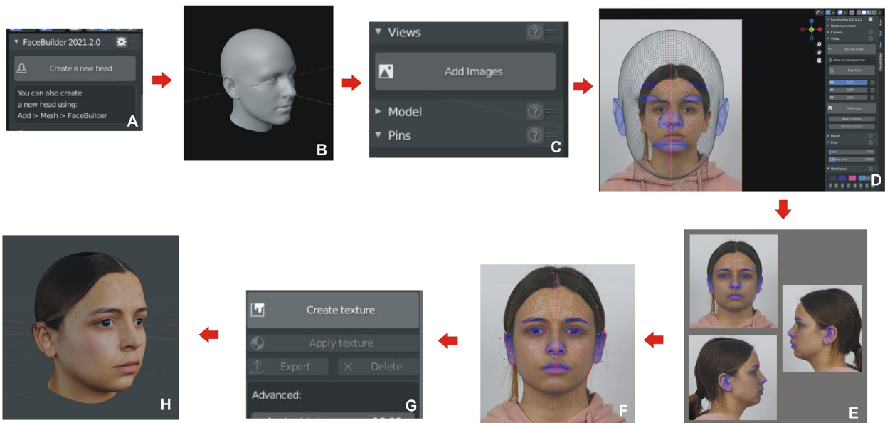
Fig 2. The steps involved in creating a 3D head model: A , Create a new head button; B , Standard 3D head model; C , Add images button; D , Align face button; E , Alignment of each of the 3 photographs with the standard head model; F , Adding additional pins to improve alignment; G , Create texture button; H , 3D reference head and face model.
